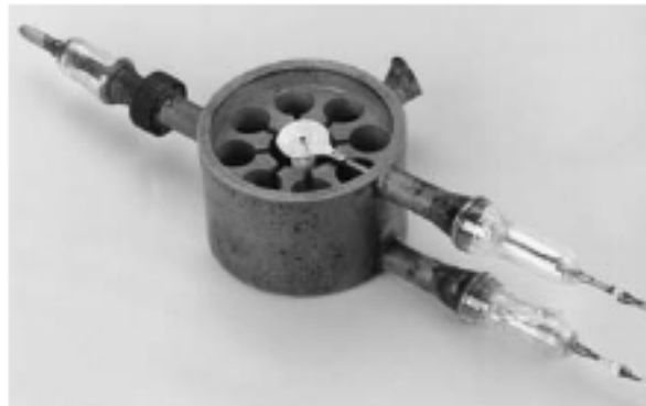
Cavity Magnetron - the world changing invention by John Randall and Harry Boot invented in 1940 (Pic. 1.11 - GEC)
