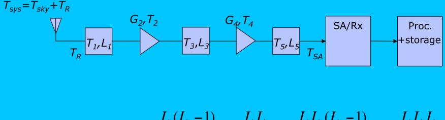
$$T_{R} = T_{1}(L_{1} - 1) + T_{2}L_{1} + T_{3}\frac{L_{1}(L_{3} - 1)}{G_{2}} + T_{4}\frac{L_{1}L_{3}}{G_{2}} + T_{5}\frac{L_{1}L_{3}(L_{5} - 1)}{G_{2}G_{4}} + T_{SA}\frac{L_{1}L_{3}L_{5}}{G_{2}G_{4}}$$
