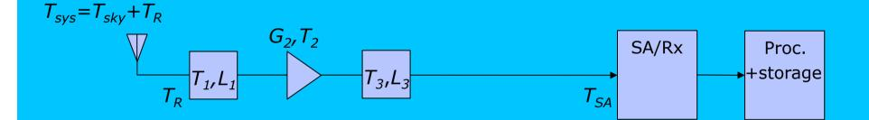
$$T_R = T_1(L_1 - 1) + T_2L_1 + T_{SA} \frac{L_1L_3}{G_2}$$
