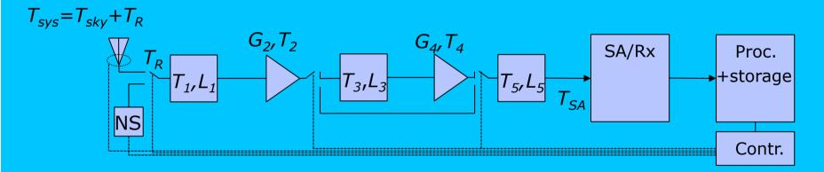
Note that in this scheme the coaxial cable attenuation and matching to the antenna is not calibrated which can give rise to ripples in the calibrated spectrum baseline.
