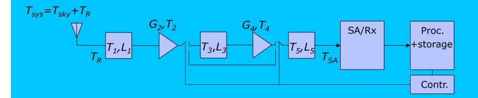
Using low-loss terminated coaxial switches to bypass an LNA that would mess up things in high signal conditions, or parts of the system that have a differing frequency range, or switch filters in and out.
