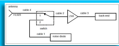
A system for 75-2000MHz. Robust and simple, yet very sensitive. Deployed in WA and SA core sites, plus a selection of 4 remote sites each.
