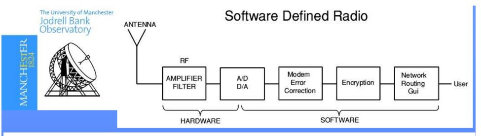
One can think of a simple ideal design for a software-defined radio in which an Analogue-to-Digital convertor (AtoD) is attached directly to an antenna, the data from which is transferred to and digitally processed in a computer to whatever format a particular application requires.
