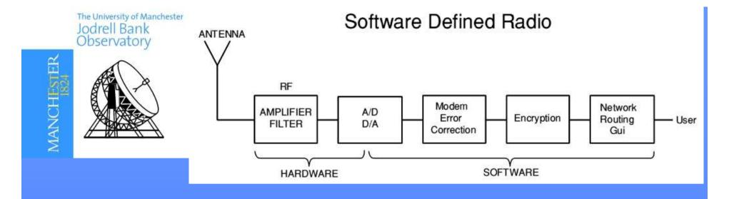
In a software defined radio communication system, many of the components normally implemented in hardware (e.g. Mixers, filters, amplifiers, modulators / demodulators, detectors etc.) are implemented by means of software running on perhaps a personal computer, or more likely on an embedded computer system (normally a real-time computing system with a dedicated function). Nowadays, these would be microcontrollers with a few designated peripherals.
