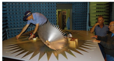
Serrated edges min. reflections
